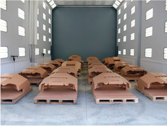
Dozens of forklift counterweights primed and ready to ship to assembly line.
