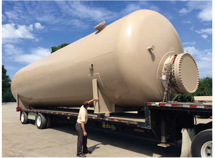
47' long tank after blast and paint for Notre Dame University.
