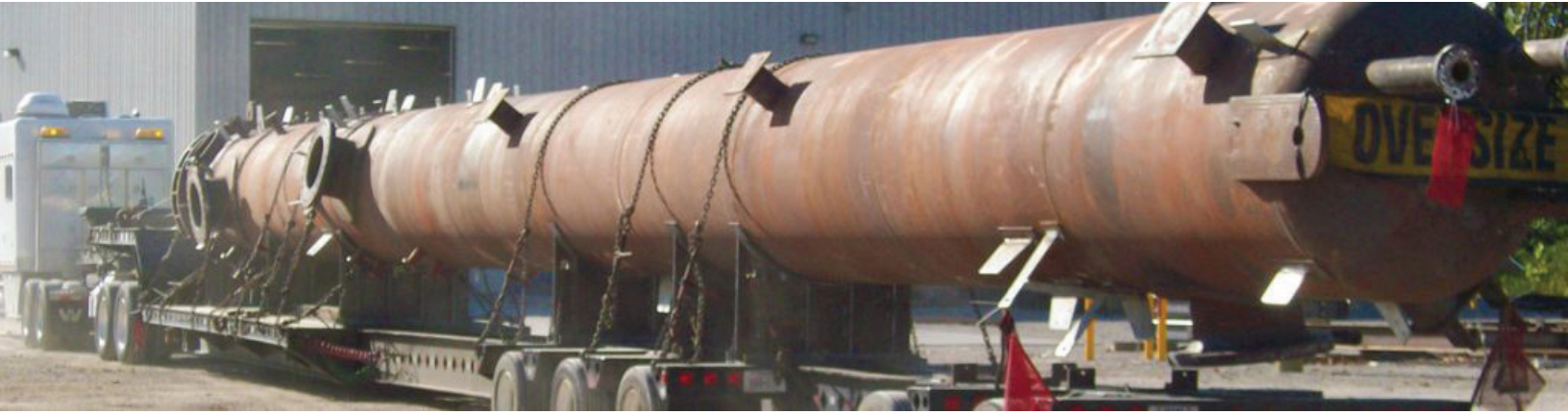
6' diameter x 100' LONG vessel for ASME stress relief at Derrick Company.
