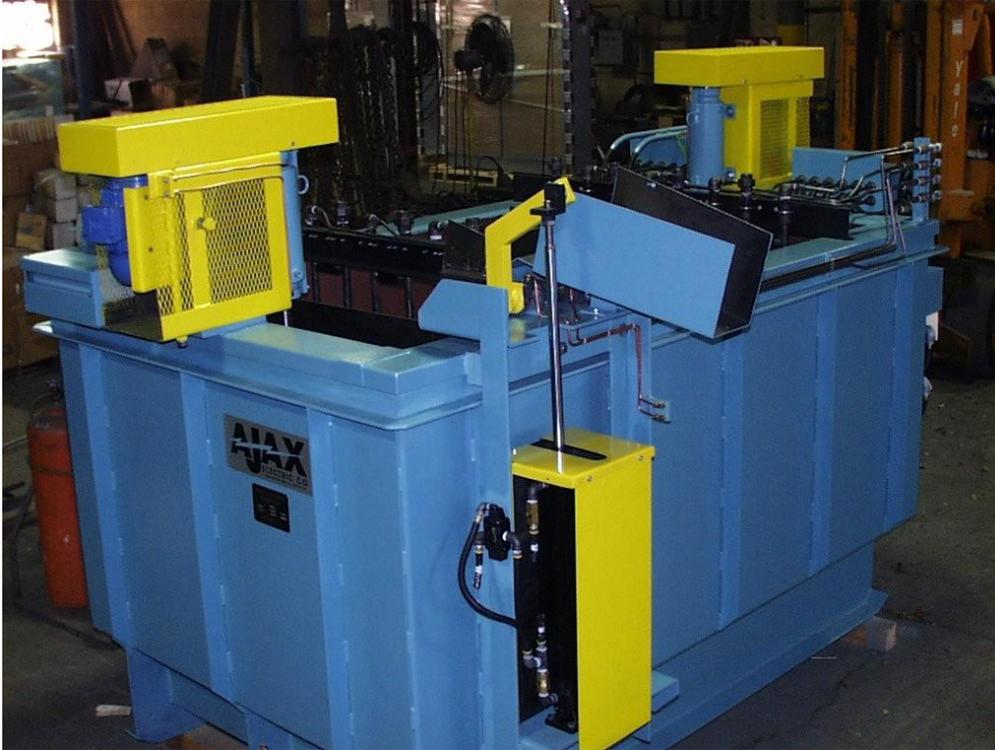
Ajax IQC-IQCR-IQCF quench furnaces may be custom engineered to meet virtually any size or production requirement, including manual or automatic operation, multiple stations, choice of filtration and cooling technologies, and integrated ECONOSAL™ salt reclamation/recovery systems. Available work-handling options include our unique UNIHOIST™ system, which may be designed for high-speed transfer of thin cross-sections or normal speed for larger (thicker) cross-sections.
