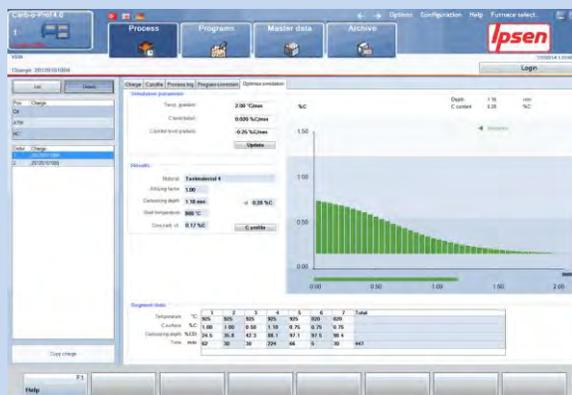
Fig. 5: Example of a simulated test run conducted using Carb-o-Prof software
