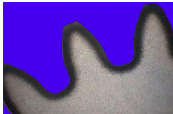
Fig. 4: Uniform surface carburizing of a gear wheel
