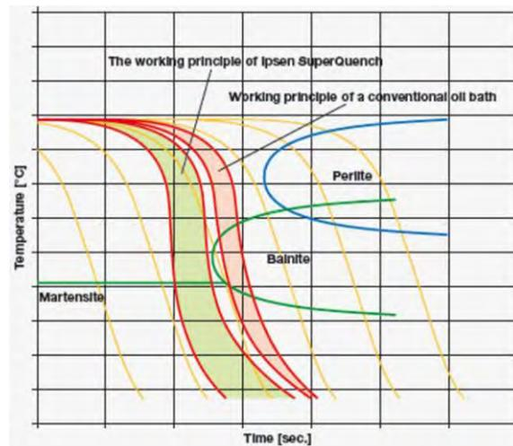
Fig. 7: Comparison of the SuperQuench® system's working principle (left) to that of a conventional oil bath (right)
