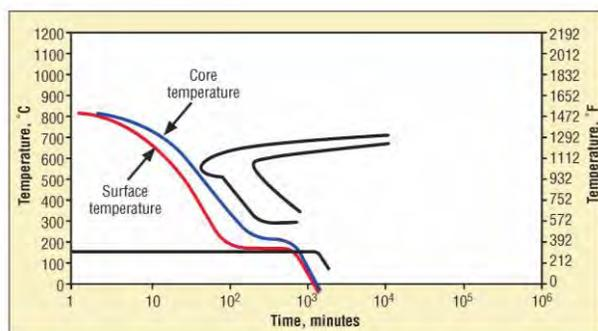
Fig. 6: Representation of an ideal cooling curve with a high cooling rate to start and a cooling rate reduction when entering the martensitic phase
