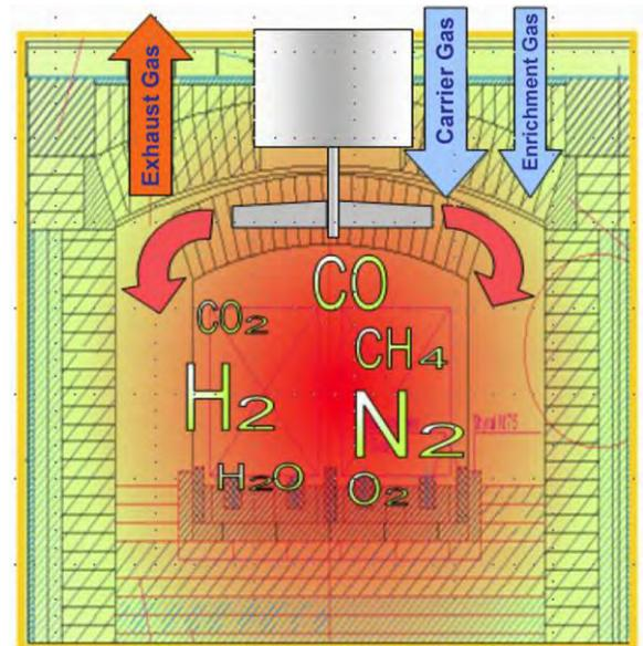
Fig. 3: A furnace atmosphere during gas carburizing
