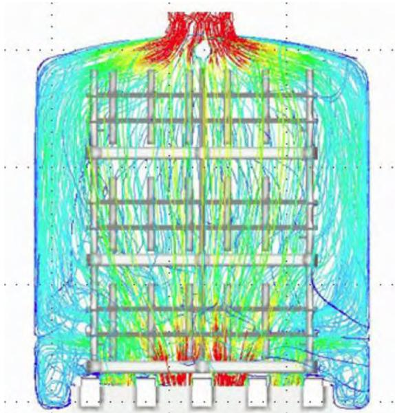
Fig. 2: Representation of the fluid flow lines in a treatment chamber
