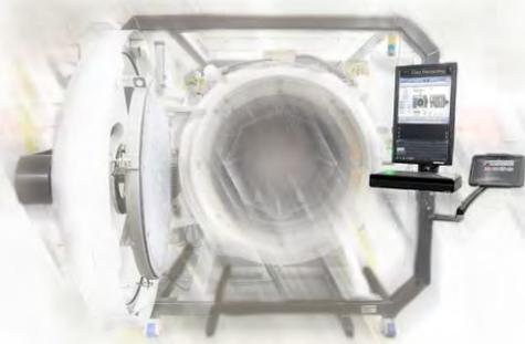
Figure 1: PdMetrics™ software platform integrated on a TITAN® 2.0 vacuum furnace.
