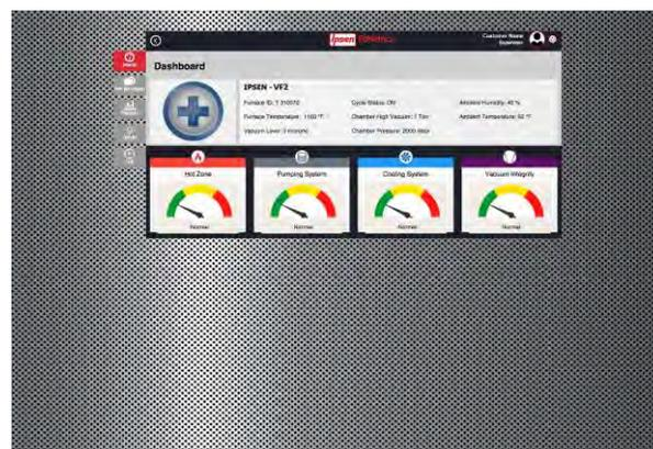
Figure 3: The PdMetrics software platform dashboard, where users can monitor the health and integrity of the hot zone, pumping system, cooling system and vacuum integrity.
