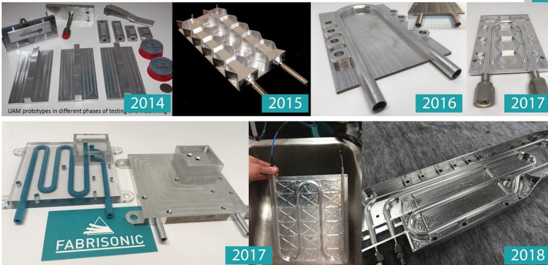
**Figure 2** - Evolution of UAM 3D printed heat exchanger with NASA JPL. Samples began small to evaluate benchmark burst and helium leak performance in 2014. The team then began focusing on technology scale-up and system integration. The culmination is a full-size functioning.
