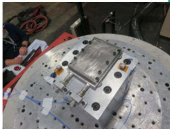
**Figure 4** - Stringent ground-based space-grade qualification testing of UAM heat exchanger devices. EWI helped Fabrisonic complete CT Scanning and helium leak testing of UAM heat exchangers throughout development.
