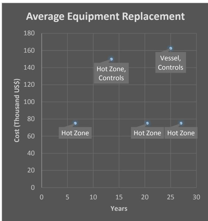
Figure 2 – The average replacement period/cost for major vacuum furnace components.
