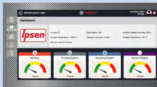
Figure 1: The PdMetrics software platform dashboard, where users can monitor the health and integrity of the hot zone, pumping system, cooling system and vacuum integrity
