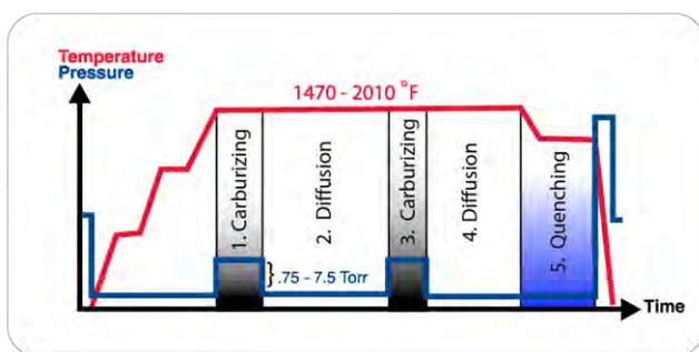
Figure 2: Typical low-pressure carburizing cycle with temperature and pressure curve
