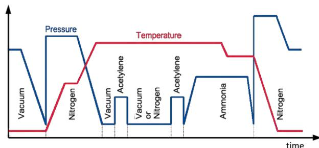
Figure 3: Typical low-pressure carbonitriding cycle with temperature and pressure curve
