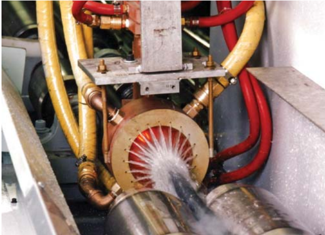
Fig. 9. Quench barrel for small-diameter, heavy-wall tubular products
