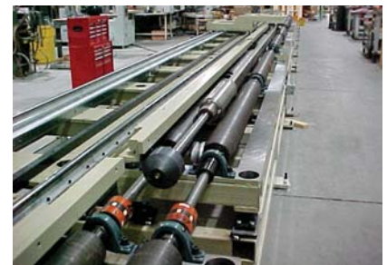
Fig. 8. Pusher-lance for precise heat treating of tubular products
