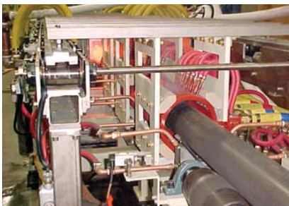
Fig. 6. Entrance end of a 40-foot horizontal scanner processing a 5 3/4-inch-diameter pipe with a 5/8-inch wall
